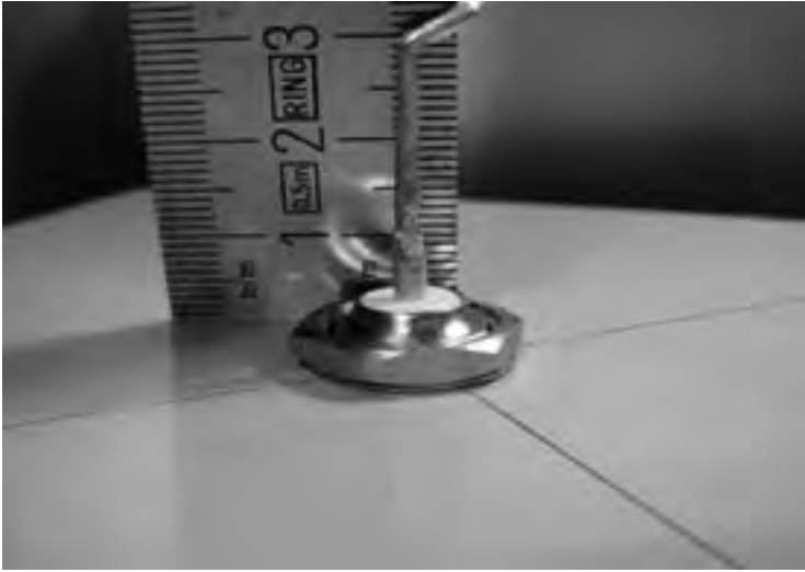
Figure 4.26: The first coil should start 3.0 cm from the surface of the plate.
