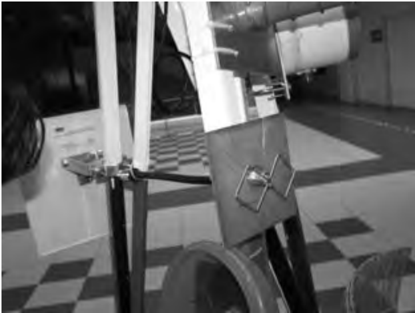
Figure 11.16: Detail of mini tower with samples of antennas, cables and pigtails.
