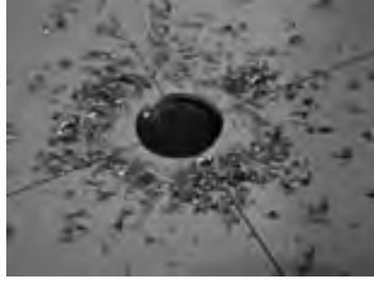
Figure 4.21: Drilling the hole in the metal plate.
