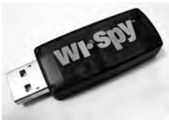
Figure 8.8: The Wi-Spy USB spectrum analyzer
