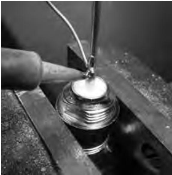
Figure 4.38: Solder the wire to the gold cup on the N connector.
