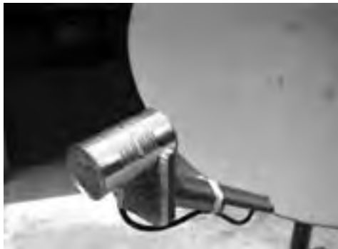
Figure 4.10: Feed horn made from a food can.
