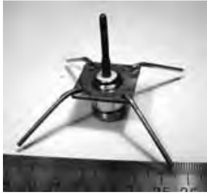
Figure 4.8: Quarter wavelength ground plane antenna.
