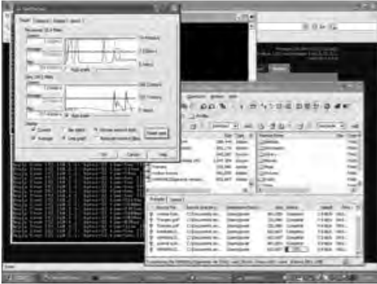
Figure 11.35: Screenshot of Javier's laptop showing details of PDF file transfer from Carlo's laptop 280 km away, using two WRT54G wireless routers, no amplifiers.
