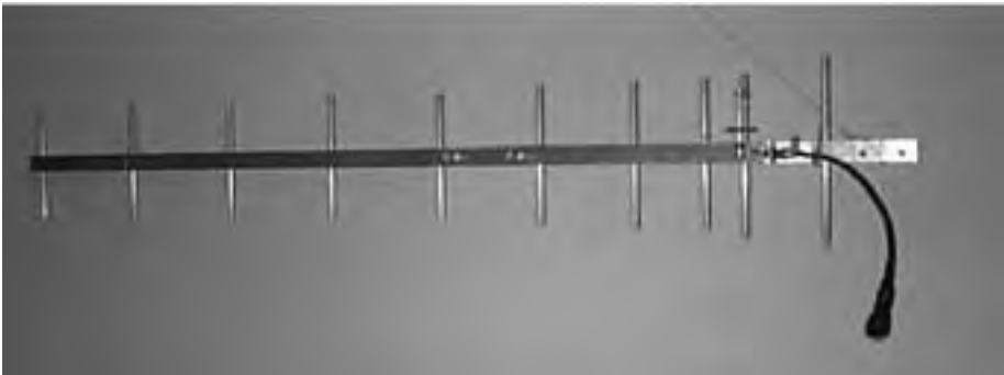
Figure 11.8: A UHF antenna for packet radio developed at ULA, LabCom.
