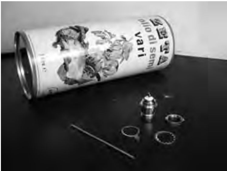
Figure 4.33: Parts needed for the can antenna.
