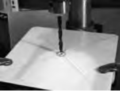
Figure 4.21: Drilling the hole in the metal plate.
