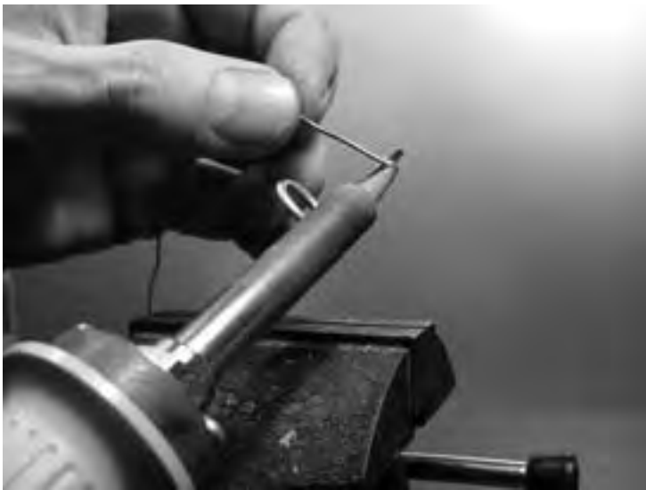
Figure 4.25: Add a little solder to the end of the wire to "tin" it prior to soldering.
