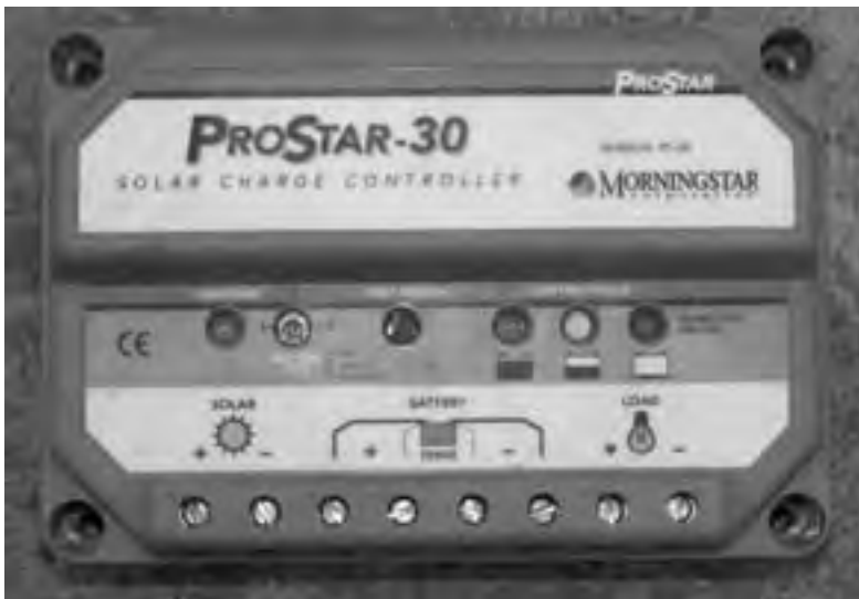
Figure 7.3: A 30 Amp solar charge controller
