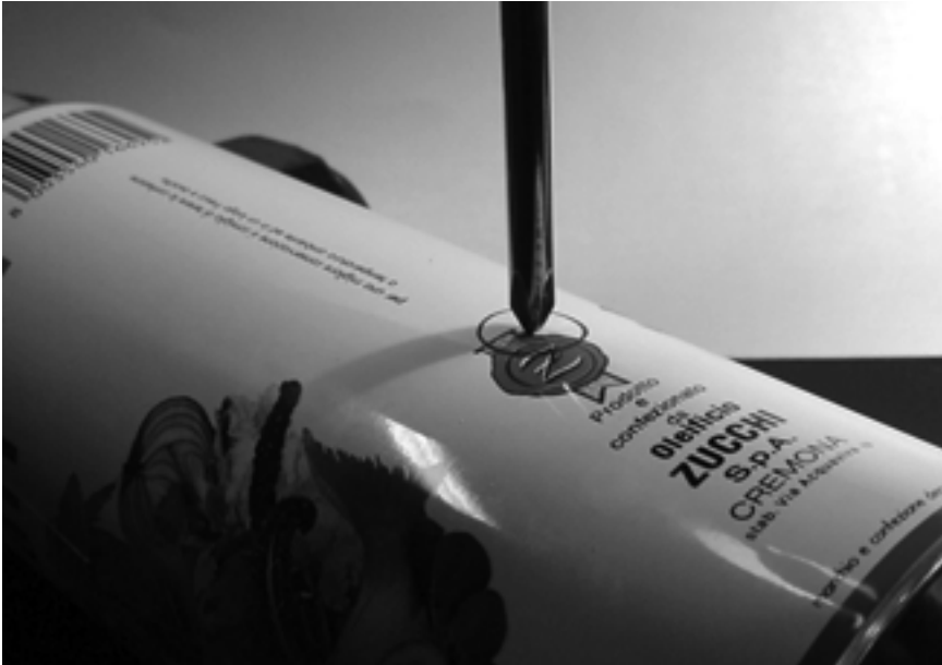
Figure 4.35: Mark the hole before drilling.
