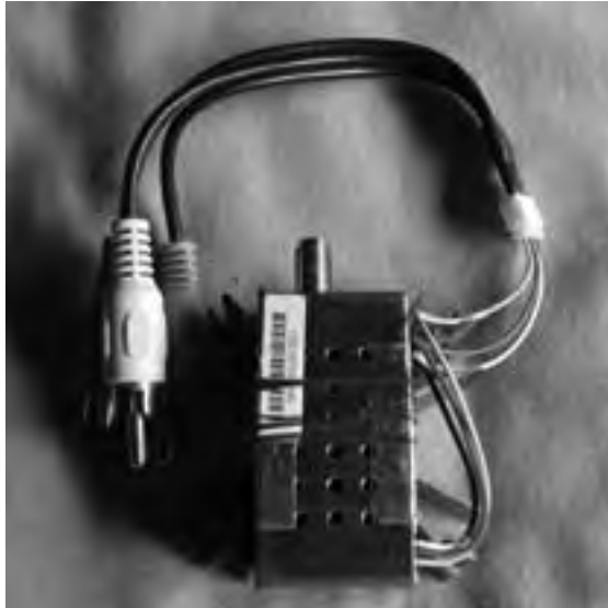
Figure 8.7: A 2.4 GHz video sender with an SMA antenna connector.
