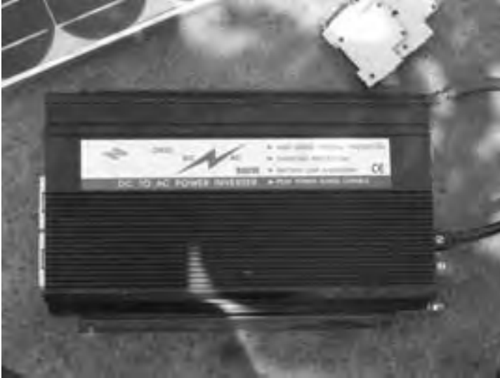
Figure 7.4: An 800 Watt DC/AC converter (power inverter)
