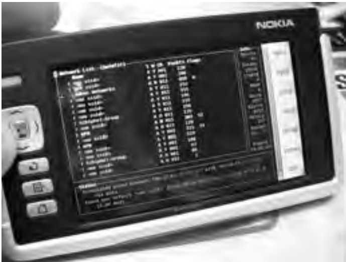
Figure 6.12: Kismet running on a Nokia 770 Internet Tablet
